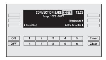
Set the timer to run the oven for 2 hours by touching the "Delay Start" control.
